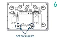
Insert cable, tighten glands and refit PCB and securing screws.
