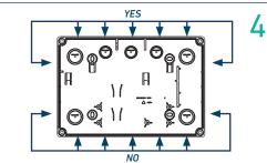
Prepare apertures (20mm knockouts) required for cable access and fit appropriate rated glands.
