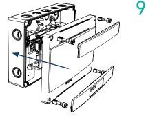
• Screw the lid to the back box using the supplied plastic screws and refit top and bottom front plastics that cover screw housings.
