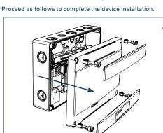
The Translator Module is IP65 rated, suitable for external mounting. The back box must be installed on the wall
